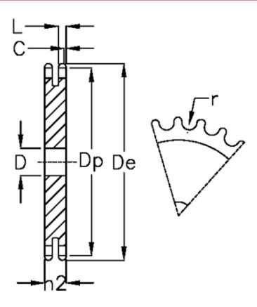
C = 2 D = 25 De = 264.5 Dp = 254.93 For chain size =  $3/4 \times 7/16$ For chain type = 12 B-2 h2 = 30.3 L = 10.8 Number of teeth = 42r = 12.07
